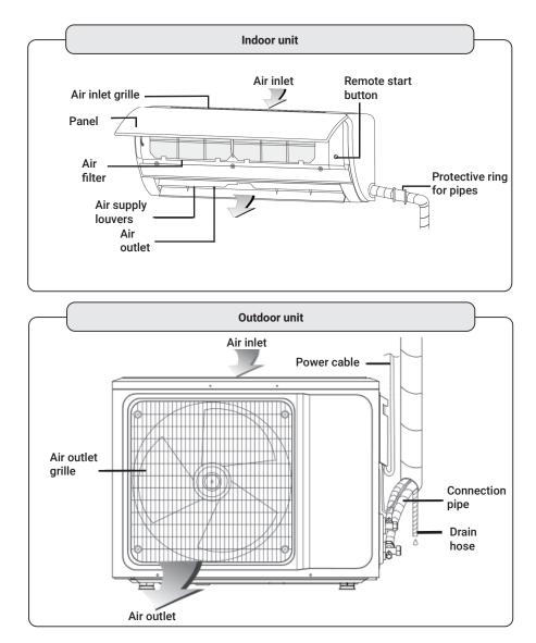
Note: All illustrations in this manual are for reference only. The actual appearance of the unit may vary. The connection diagram depends on the air conditioner model.
